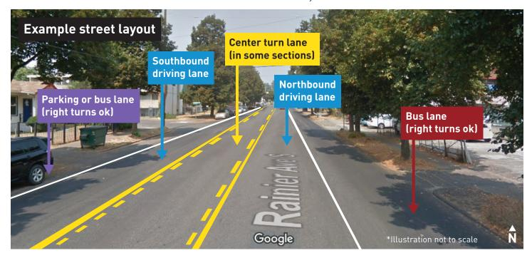
The street layout concept we're studying typically includes a parking lane (either on the west or east side of the street), one driving lane in each direction, center turn lane, and bus lanes. Some sections will include a southbound bus lane in place of the parking lane. During fall 2018 and early 2019, we're reaching out to adjacent neighbors to get input on safety improvements and changes to the street layout. Please contact us to share your input.
