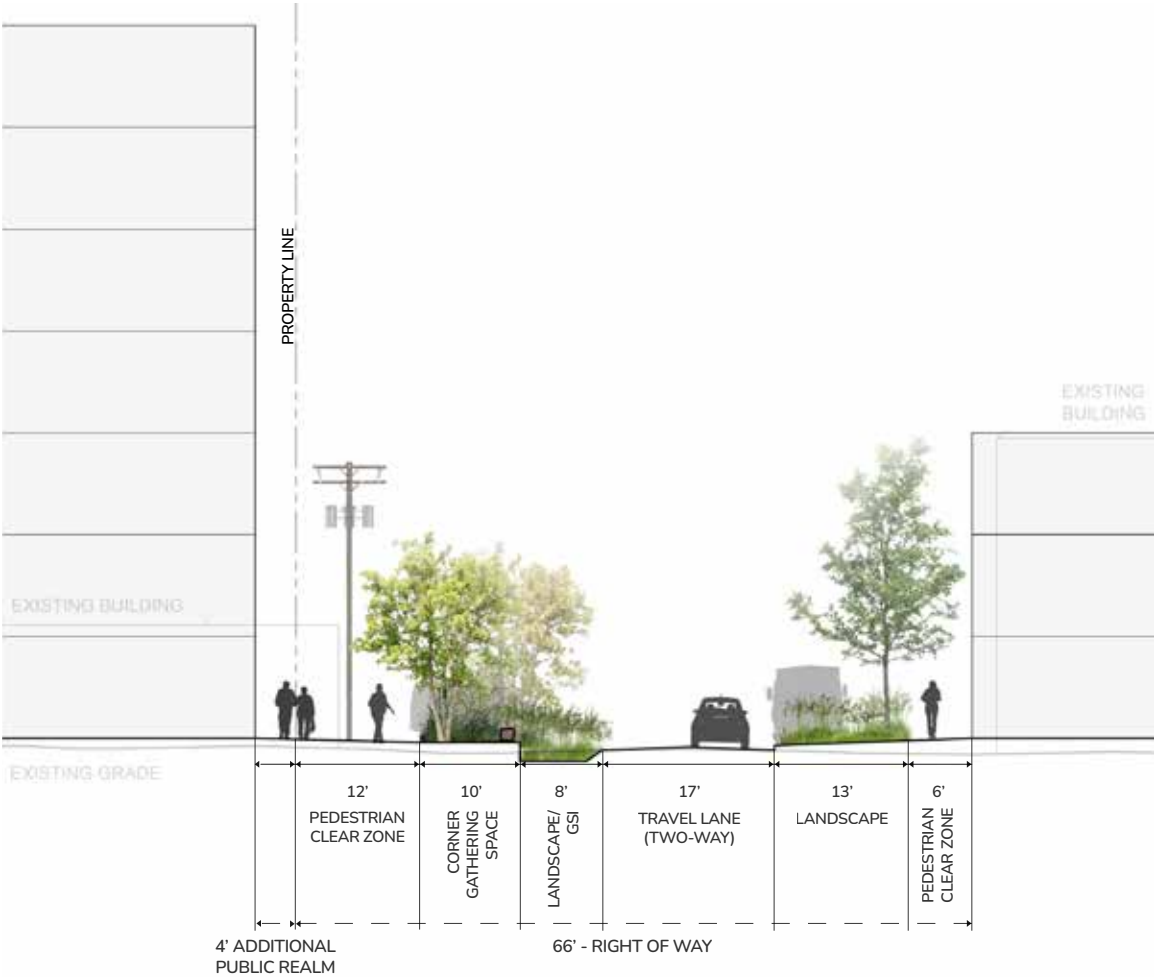
Proposed 5th Ave S section (B) looking north at a corner eddy.
