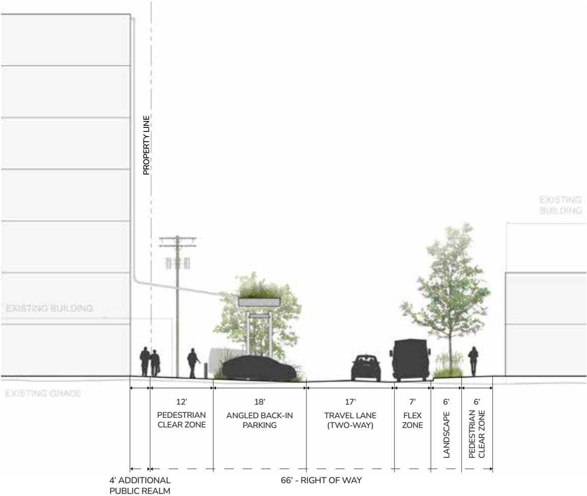
Proposed 5th Ave S section (A) looking north at angled back-in parking.
