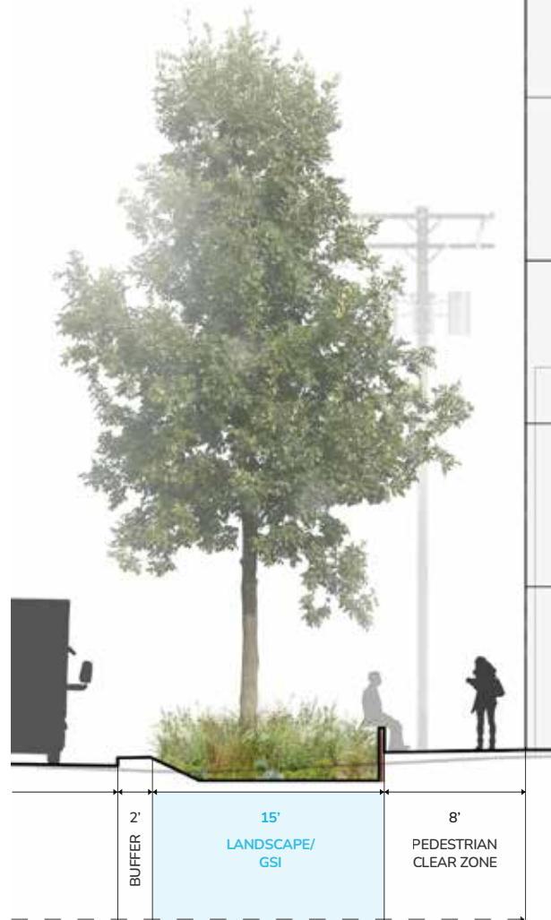
Left: proposed 4th Ave S section looking north, showing bioretention cells.
