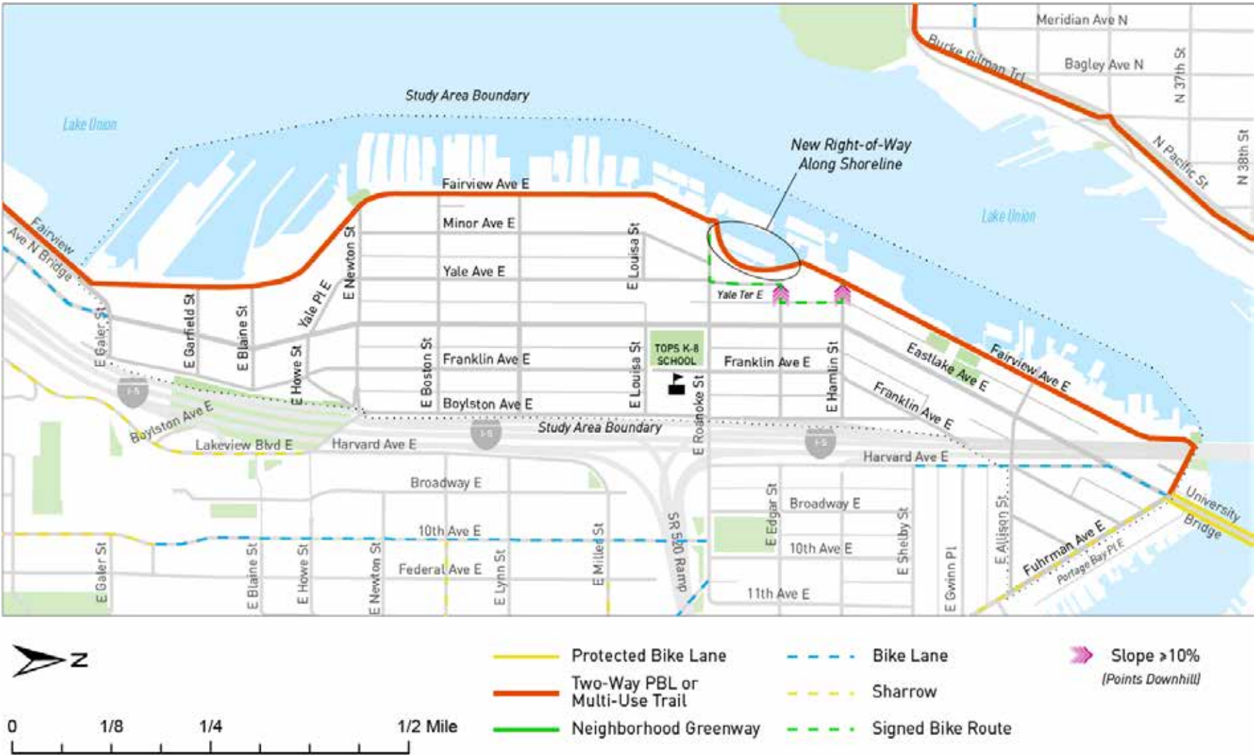
Figure 5-11. Option 6: Multi-Use Trail on Fairview Ave E Option 6 would add a multi-use trail on the west side of Fairview Ave E throughout the study area. This option includes a multi-use trail in new right-of-way along the Lake Union shoreline between E Hamlin St and E Roanoke St to provide a flat and continuous bike route. This would require right-of-way acquisition along about 740 feet of the shoreline. This option would not add bicycle facility improvements on Eastlake Ave E between the University Bridge and the Fairview Ave N bridge.
