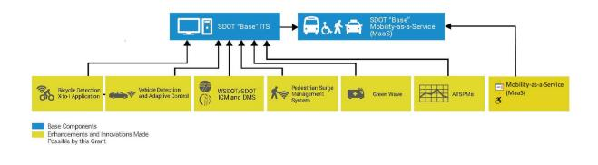
**Base ITS.** SDOT has programmed funds to install systems to address the major and unpredictable congestion in the UW subarea. Core systems to be installed as part of Base ITS include:
