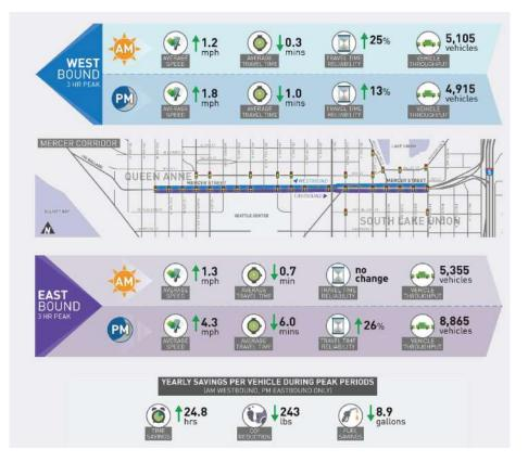
Figure 11: Adaptive Control Measured Improvements in the Mercer Corridor
