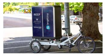
Electric pallet used for goods delivery. Photo source: UW Freight Lab
