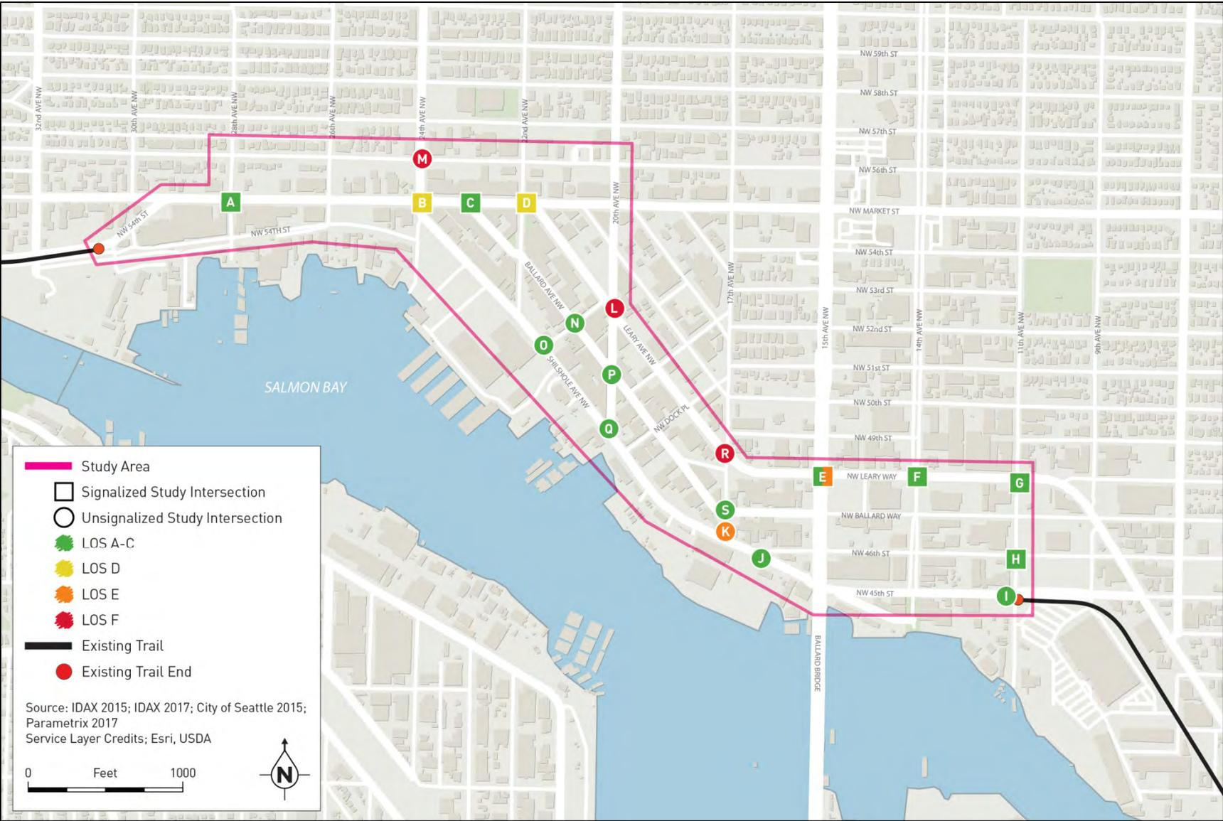
Figure 7-3. Existing Conditions PM Peak Hour Study Intersection Level of Service
