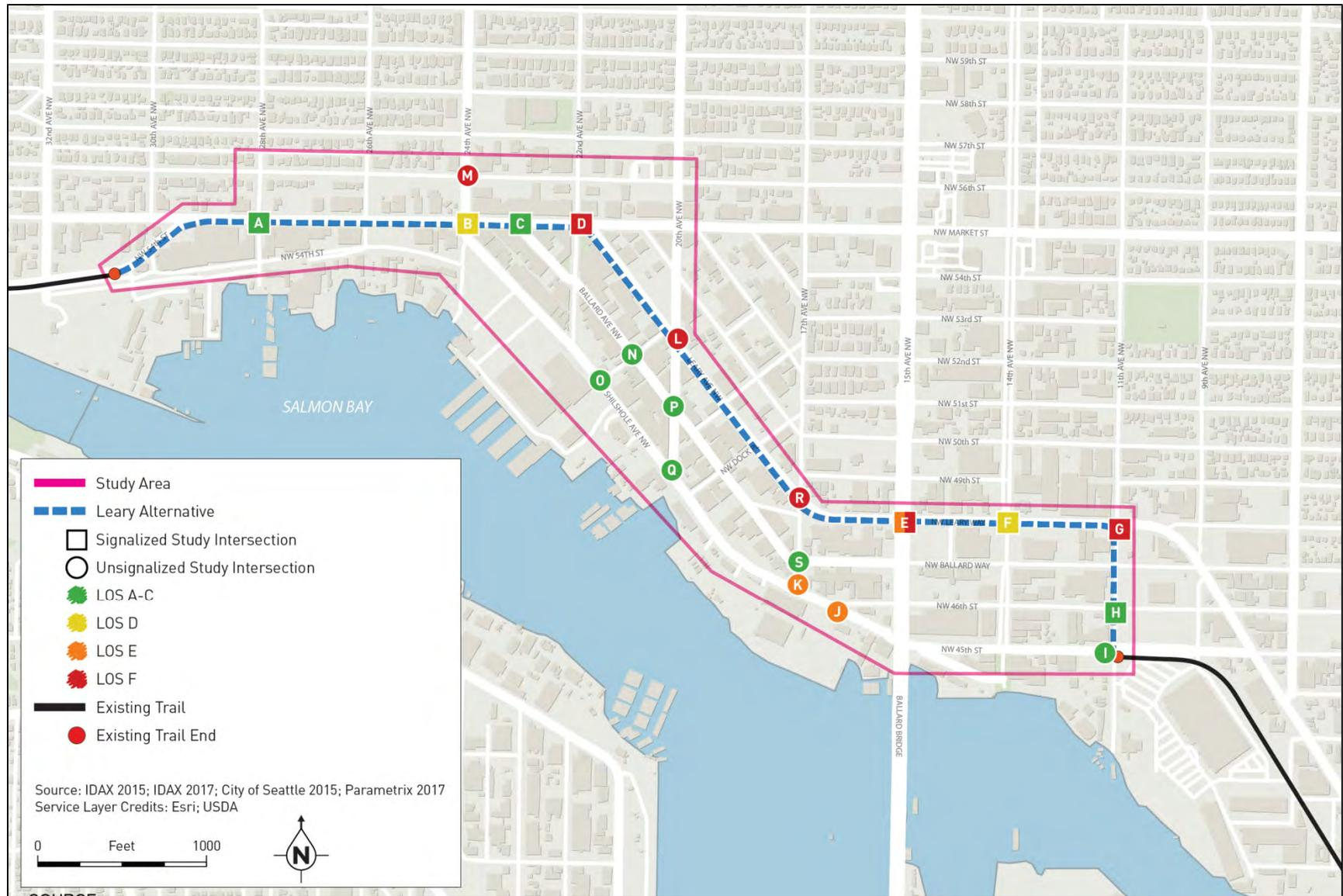
Figure 7-16. Leary Alternative PM Peak Hour Study Intersection Level of Service
