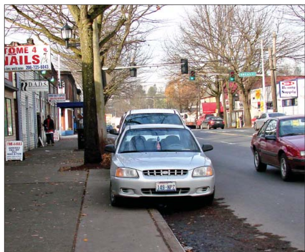
Drivers often park partially on the planting strip due to the perceived narrow lane widths.
