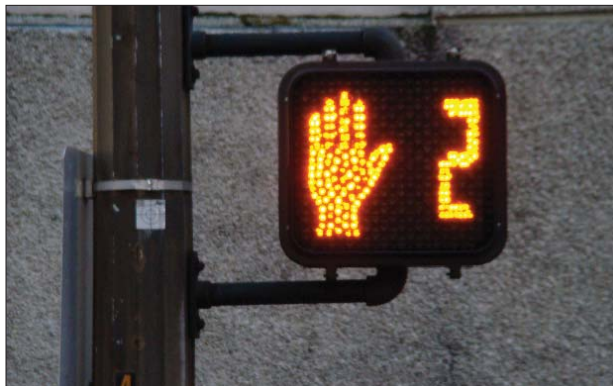
A countdown signal alerts pedestrians to how much time remains for them to cross the street safely.
