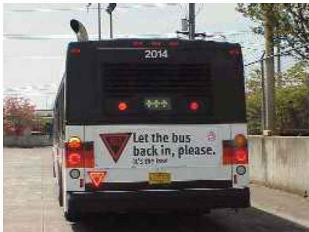
"Yield" sign illuminates as bus driver moves back into traffic lane. See Recommendation T66.
