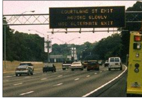
Figure A-6: Variable Message Sign
