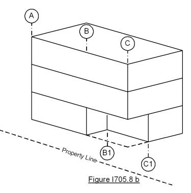
Note: Opening protection in wall C to C1 isn't considered in Figures 1705.8a and 1705.8b because it is perpendicular to the property line.
