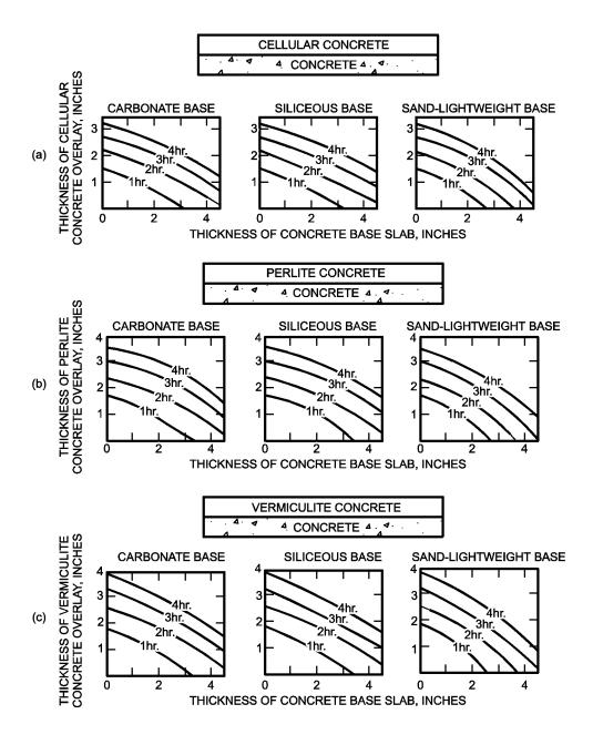
FIGURE 722.2.3(1) FIRE-RESISTANCE RATINGS FOR CONCRETE ROOF ASSEMBLIES
