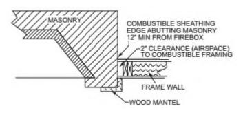
FIGURE 2113.19 ILLUSTRATION OF EXCEPTION THREE CHIMNEY CLEARANCE PROVISION
