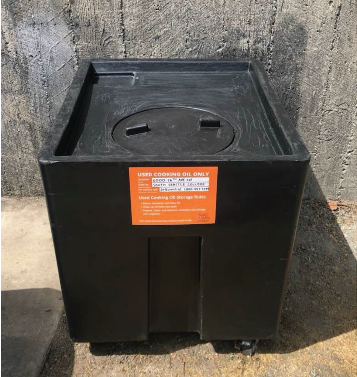
Figure 2. Example of a labeled used cooking oil tote located on a level surface with a secure lid. (New Figure)
