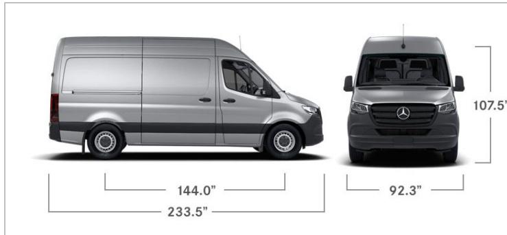
Figure 12: Design Vehicle 1 (High-roof Sprinter Van)
