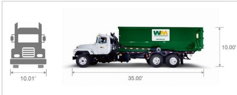
Figure 14: Design Vehicle 2 (Roll-off Waste Collection Truck)
