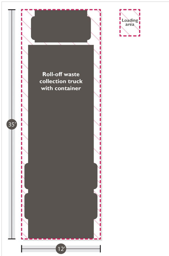
Figure 15: Recommended Off-street Loading Area for Design Vehicle 2
