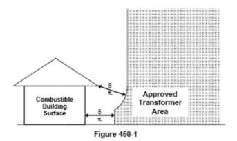
(2) A transformer installed adjacent to a building or structure with no combustible surface shall be located no closer than 610 mm (2 ft) to the building or structure and shall be outside a line extended vertically from the ends of the eaves or rooflines as illustrated in the shaded "Approved Transformer Area" shown in Figure 450-2.
