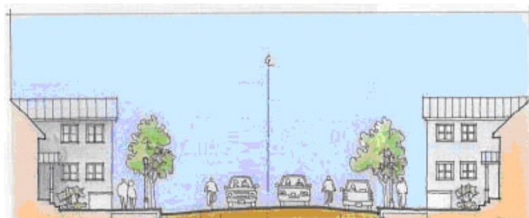
A-2: Minor grade separations create residential privacy, and provide opportunities for front porches and stoops.
