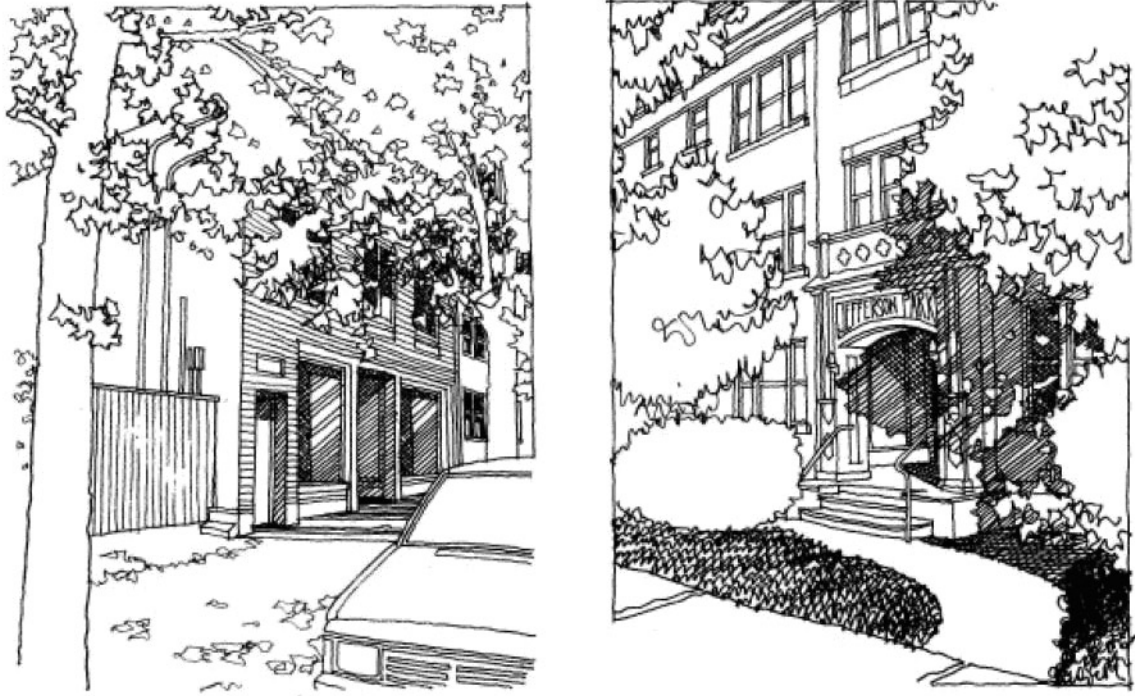
C-1: Simple massing oriented to the street provides visual relief with a facade that exhibits pleasing proportions, recessed windows and entries created with modulation, fenestration pattern and shadow lines. A classic, well marked and articulated brick building oriented to public space on Beacon Hill.
