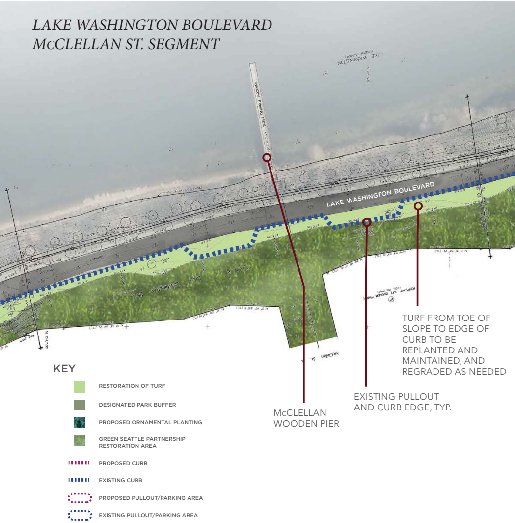
FIGURE 6.8: PROPOSED RESTORATION SITE PLAN (McCLELLAN ST.)
