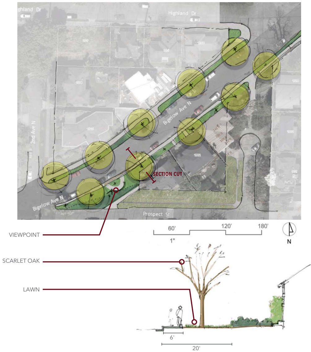
FIGURE 10.4: PROPOSED REHABILITATION PLAN & SECTION FOR QUEEN ANNE BOULEVARD
