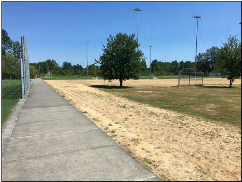
View east along the south edge of Field 6, toward Field 7, showing the grade relationship of these two existing fields. They are also on the same plane, although sloping collectively at 0.5% to the east.
