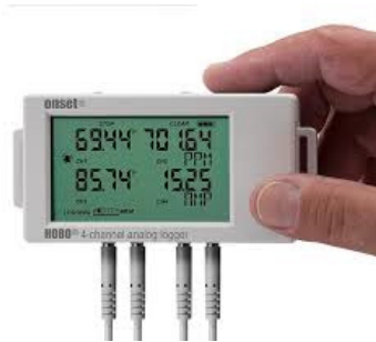
4-channel logger with external sensors
