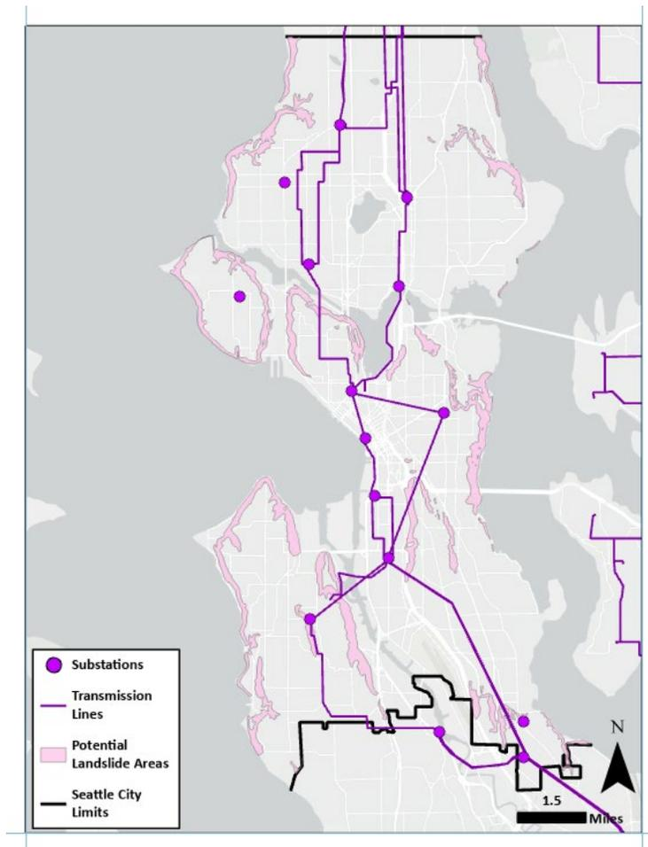
Notes: This map overlays potential landslide areas with substations and transmission lines in Seattle. Two substations border potential landslide risk areas (City of Seattle, 2022; U.S. Energy Information Administration, 2020).
