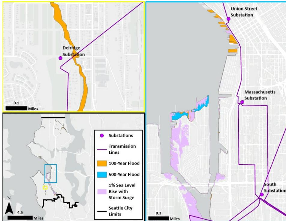
Notes: This set of maps overlays the 100-year and 500-year floodplains and likely 2050 sea level rise of 3.1 feet (using a 1% likelihood scenario and including storm surge). Inset maps indicate areas where the Delridge substation and Union Street Substation are near the 500-year floodplain (City of Seattle, 2022; Miller et al., 2018; National Oceanic and Atmospheric Administration, 2021; Roop et al., 2018; U.S. Energy Information Administration, 2020).
