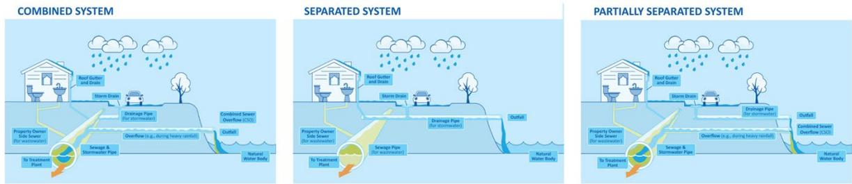
**Figure 32. Types of Sewer Systems in Seattle**
