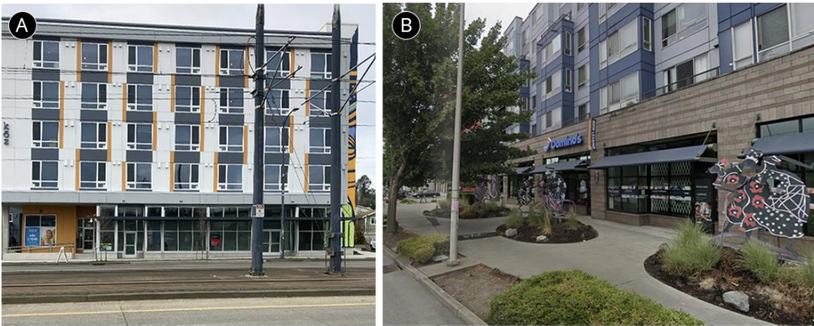
Mixed-Use/Commercial Frontage Conditions: (A) A new mixed-use development with zero setback and high ground-floor transparency, (B) A mixed-use development incorporating deeper setbacks, landscaped buffers, public art weather protection, and active commercial frontages (Framework 2025).
