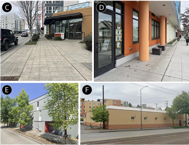
Private Frontage Conditions: (C) Residential development with a deep setback paved as a plaza, but lacking seating, bike racks, or other pedestrian amenities. (D) Residential ground floor with minimal setbacks, low transparency, and street trees along the curb. (E) Residential development with direct unit entries to the street. The facade incorporates very low transparency but varied materials, facade articulation, and a street tree buffer. (F) The Filipino Community Center incorporates modulation and more windows on a secondary frontage, but the MLK frontage has high windows and low transparency, creating a more closed edge (Framework 2025).
