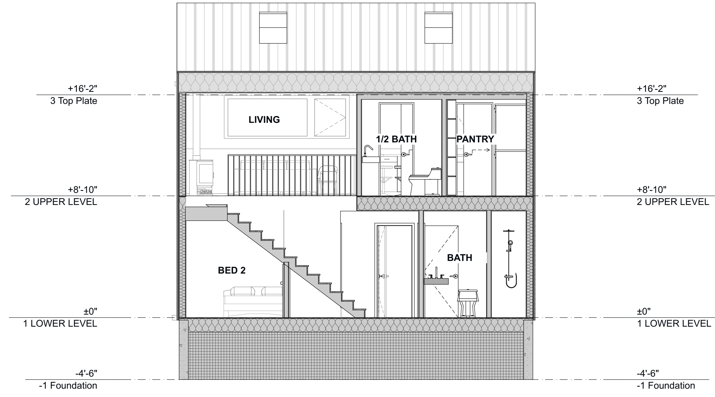
2 Section at Stair Looking South A301 SCALE: 1/4" = 1'-0"
