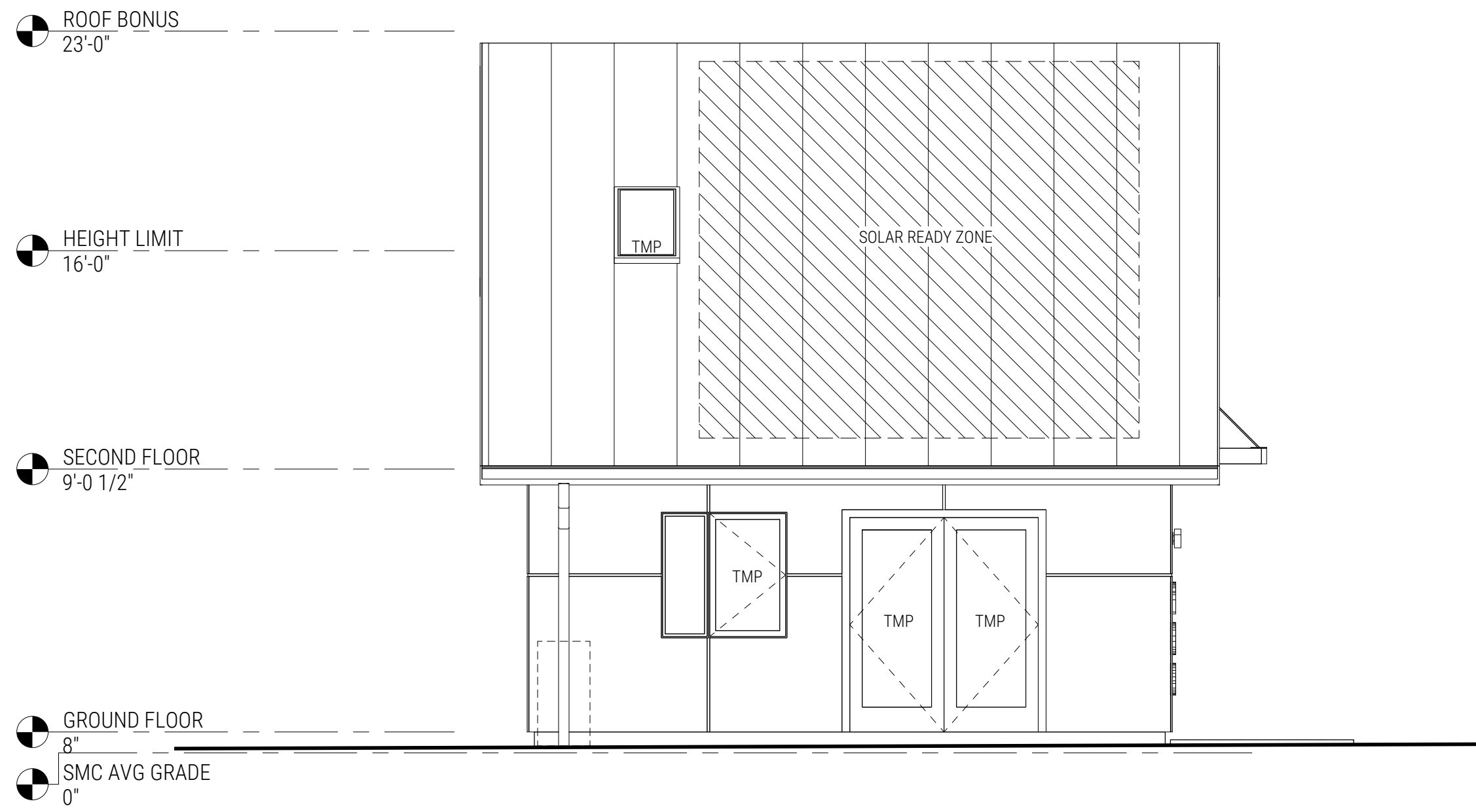
② WEST ELEVATION 1/4" = 1'-0"
