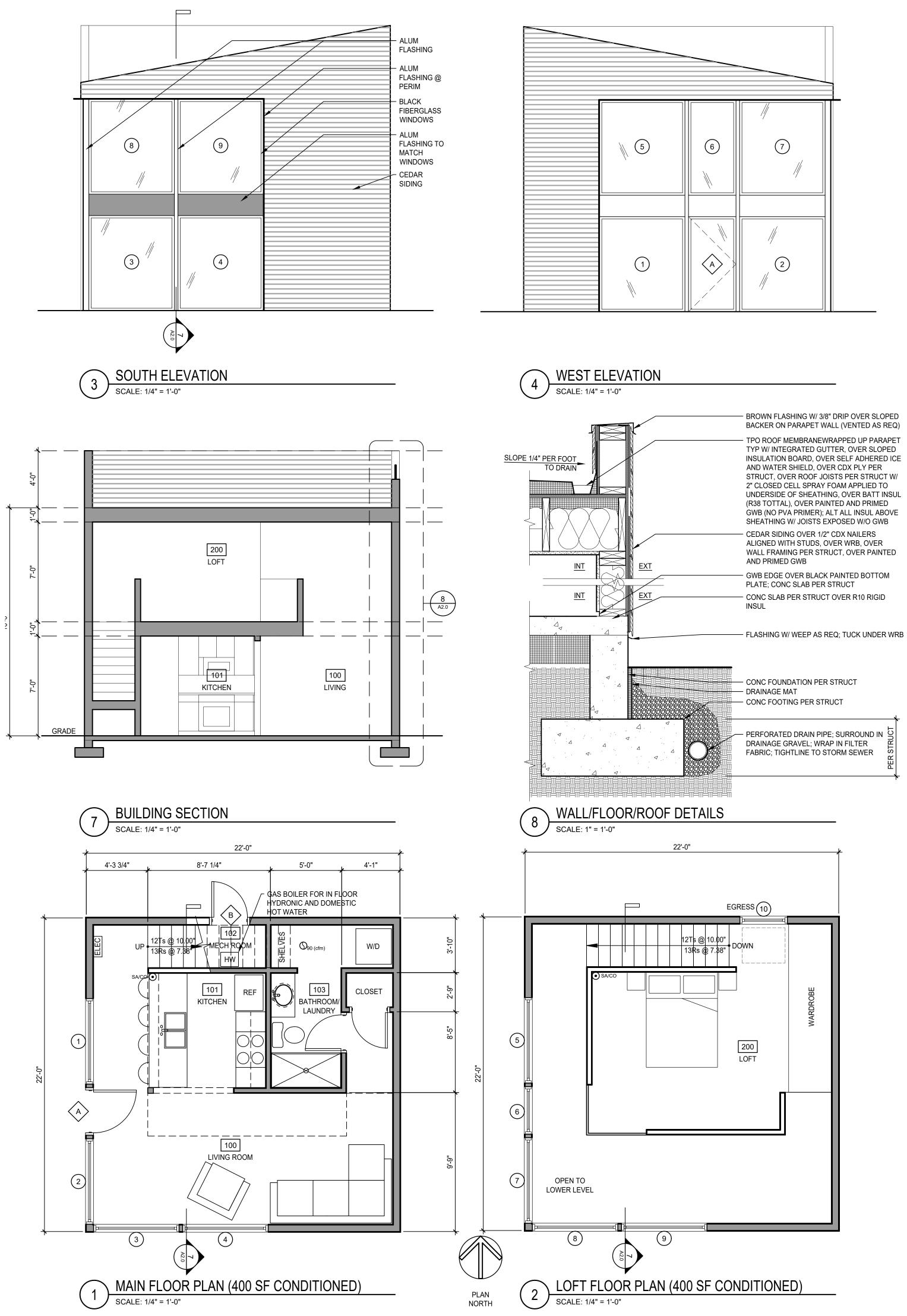
TPO ROOF MEMBRANEWRAPPED UP PARAPET TYP W/ INTEGRATED GUTTER, OVER SLOPED INSULATION BOARD, OVER SELF ADHERED ICE AND WATER SHIELD, OVER CDX PLY PER STRUCT, OVER ROOF JOISTS PER STRUCT W/ 2" CLOSED CELL SPRAY FOAM APPLIED TO UNDERSIDE OF SHEATHING, OVER BATT INSUL (R38 TOTTAL), OVER PAINTED AND PRIMED GWB (NO PVA PRIMER); ALT ALL INSUL ABOVE SHEATHING W/ JOISTS EXPOSED W/O GWB
