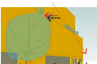
Consider setting back the upper level to reduce shadows and increase solar access at street level.
