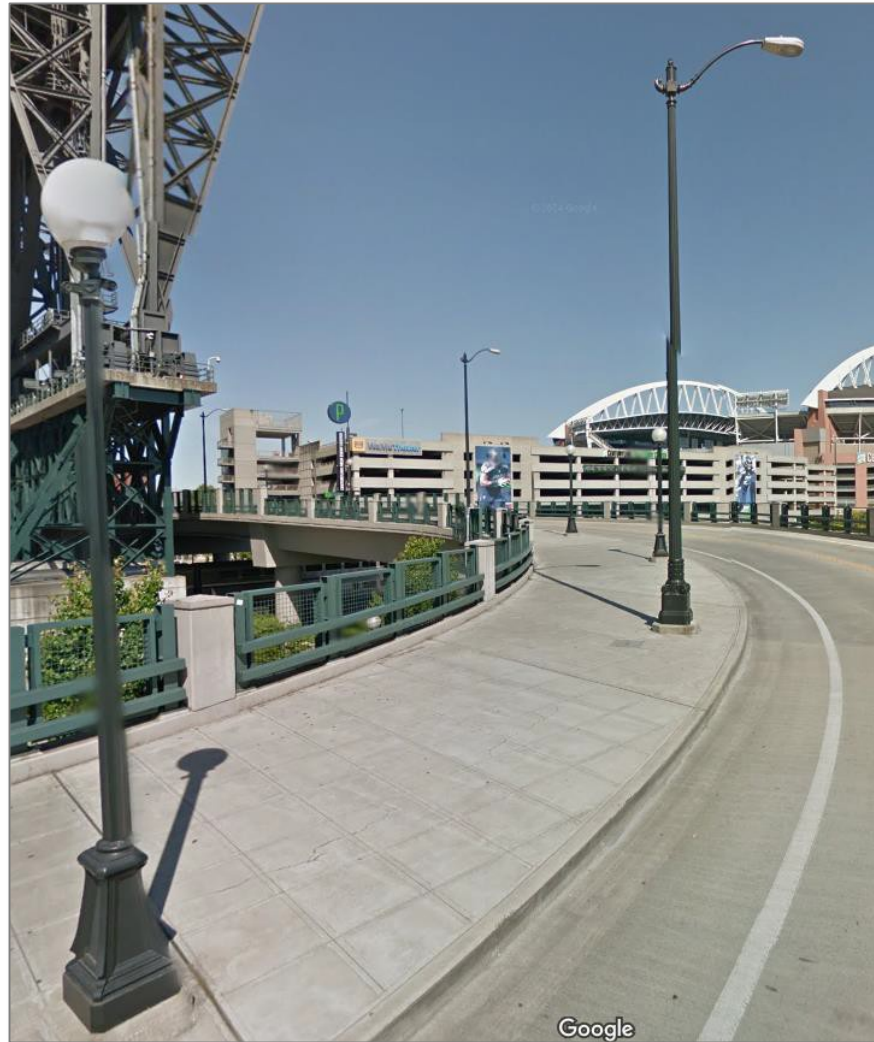
Example of cobra heads and pedestrian lighting intermixed 20
