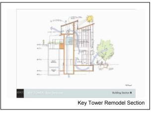
The structure is essentially in three pieces: the elevator core and two columns. These elements support the glass which will be pristine, a triangle that's glazed—it will be a plane lit with ambient light off the
