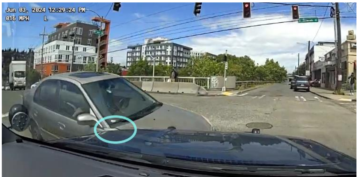
ICV image immediately after impact. Hood gap on Vehicle #1's is no longer level.
