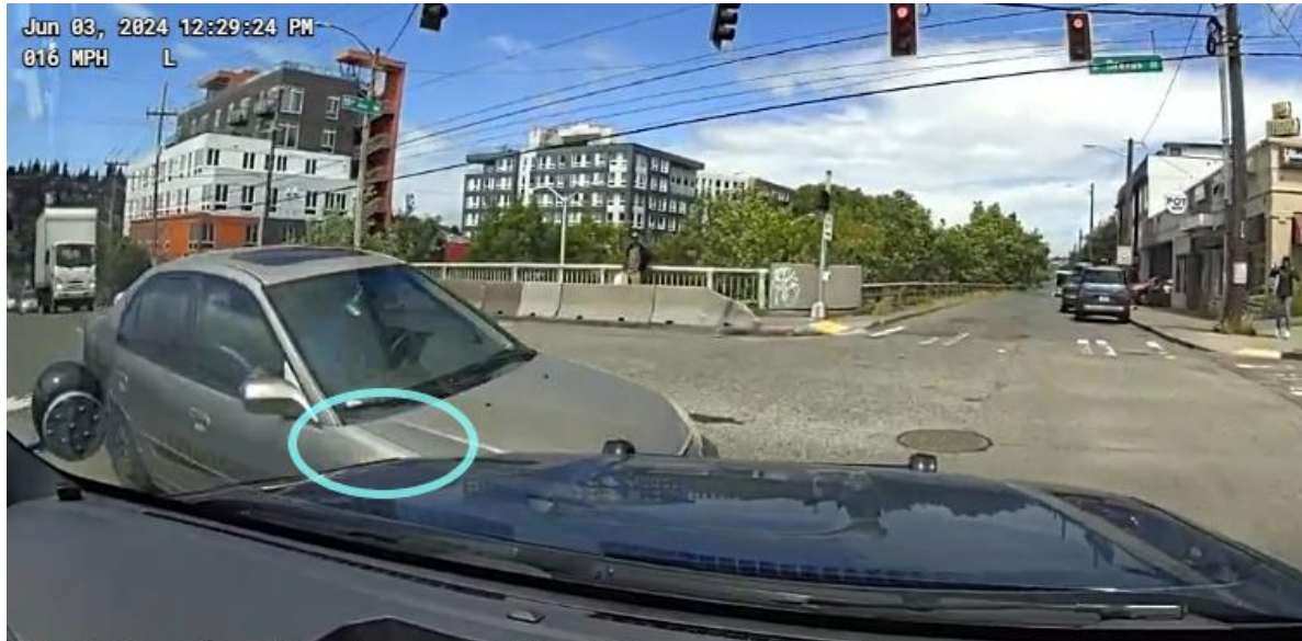
ICV image immediately prior to impact. Hood gap on Vehicle #1, circled in blue, is level.
