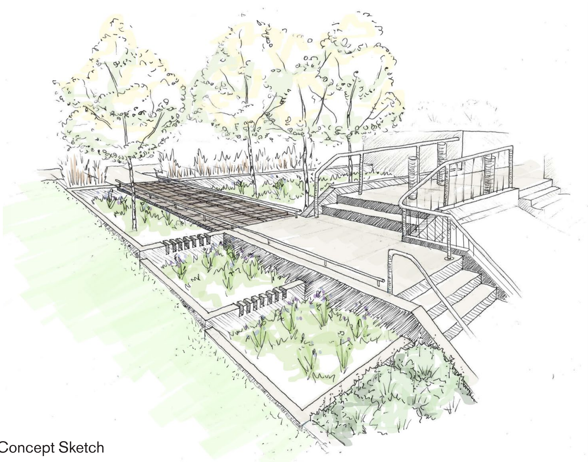
The pedestrian experience at the corner of Eastlake Ave E and Fairview Ave N is enhanced by bioretention planters. The terraced planters detain stormwater from the new parking garage and flow into one another via functional weirs. A grated walkway extends over the first planter in the series of three, providing access to the parking garage and concrete stairs down to Fairview Ave N.
