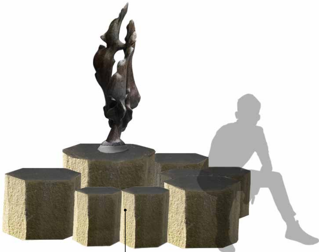
BASALT COLUMNS - LARGE STONE - CLUSTER OF 8' TO 9' WIDTH - CLUSTER OF 8' TO 9' LENGTH - 1'-6" TO 2'-6" TALL - SECTION CUTS WITH HONED/POLISHED FINISH
