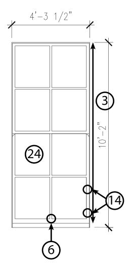
Lower sash is loose within frame and rattles with air movement
