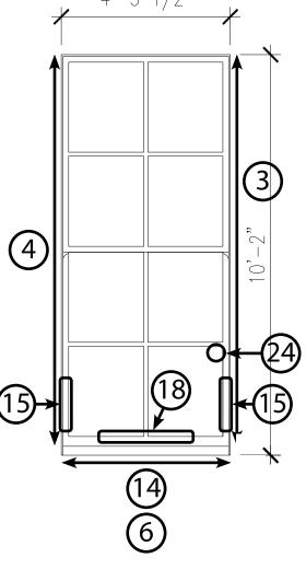
Interior plexiglass guard fastened to lower sash
