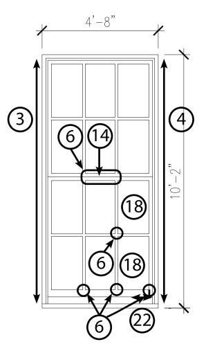
Interior plexiglass guard fastened to lower sash
