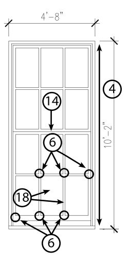
Interior plexiglass guard fastened to lower sash
