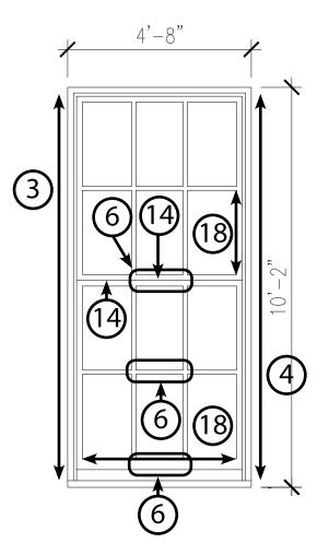
Interior plexiglass guard fastened to lower sash
