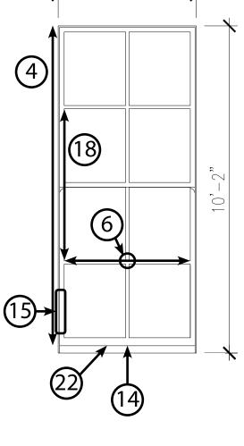
Interior plexiglass guard fastened to lower sash
