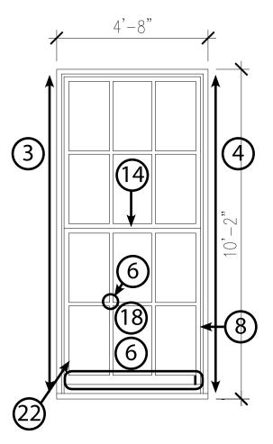
Interior plexiglass guard fastened to lower sash
