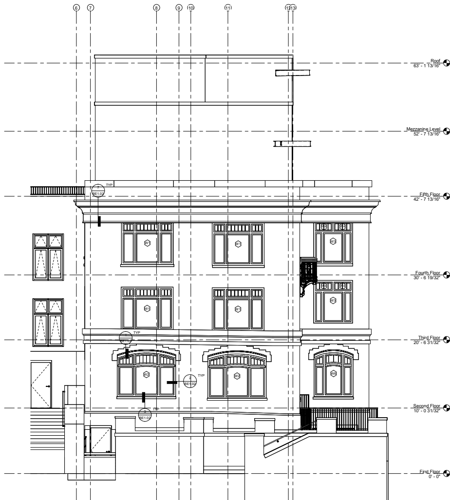
① WEST ELEVATION 1/4" = 1'-0"
