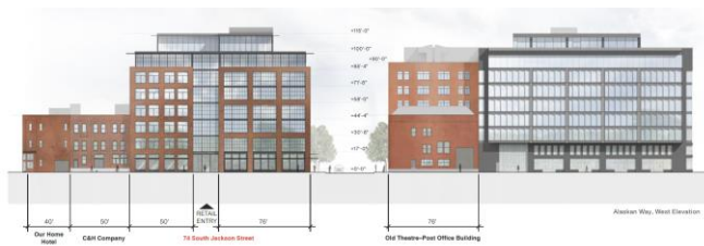
Figure xxx. An example of height analysis from a viewpoint looking into the district. Note how the building façade on the left is divided into different sections to reduce its visual massing while the new building on the extreme right does not address this objective.
