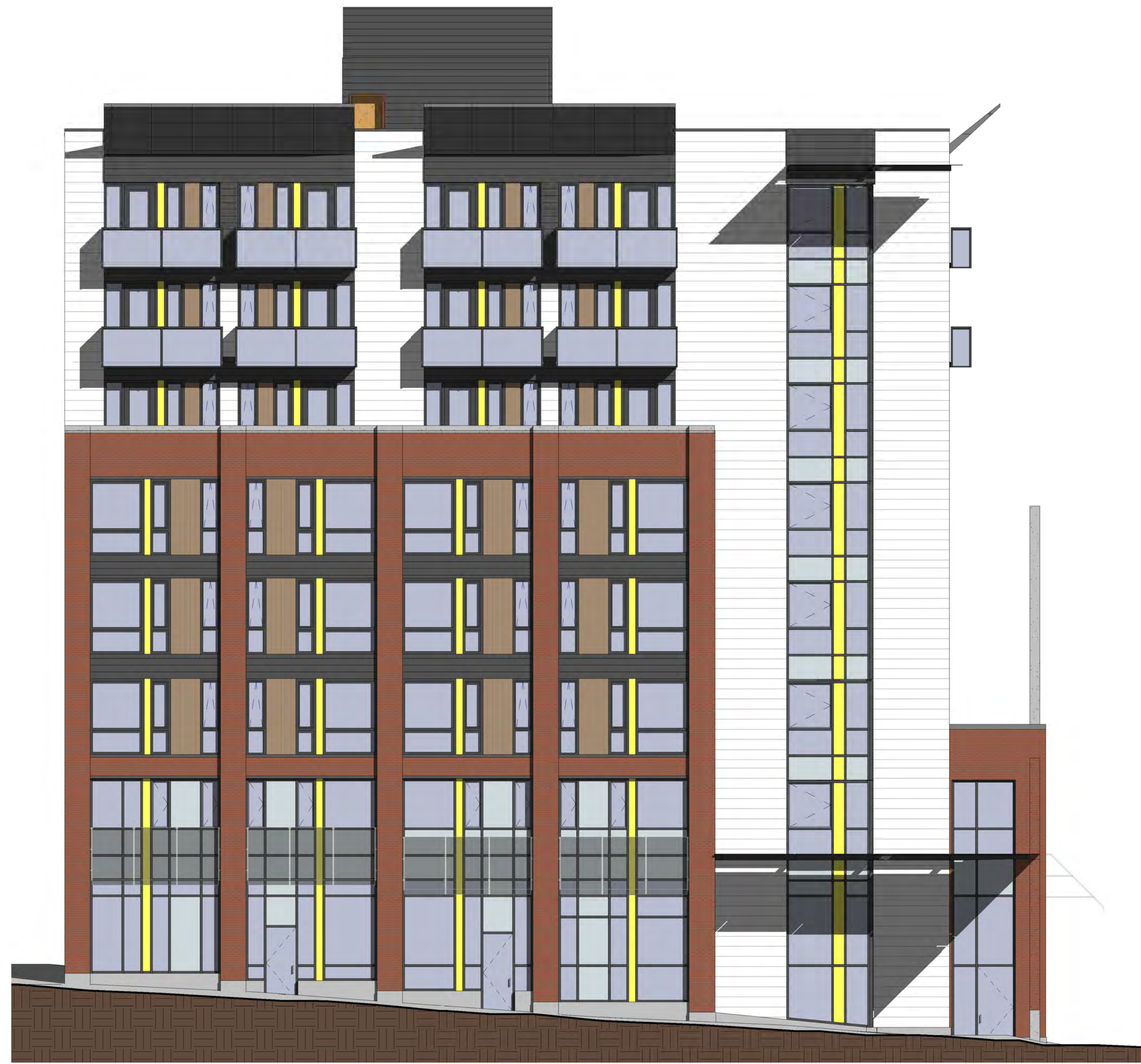
2 ELEVATION - NORTH FACADE SCALE: 1/8" = 1'-0"
