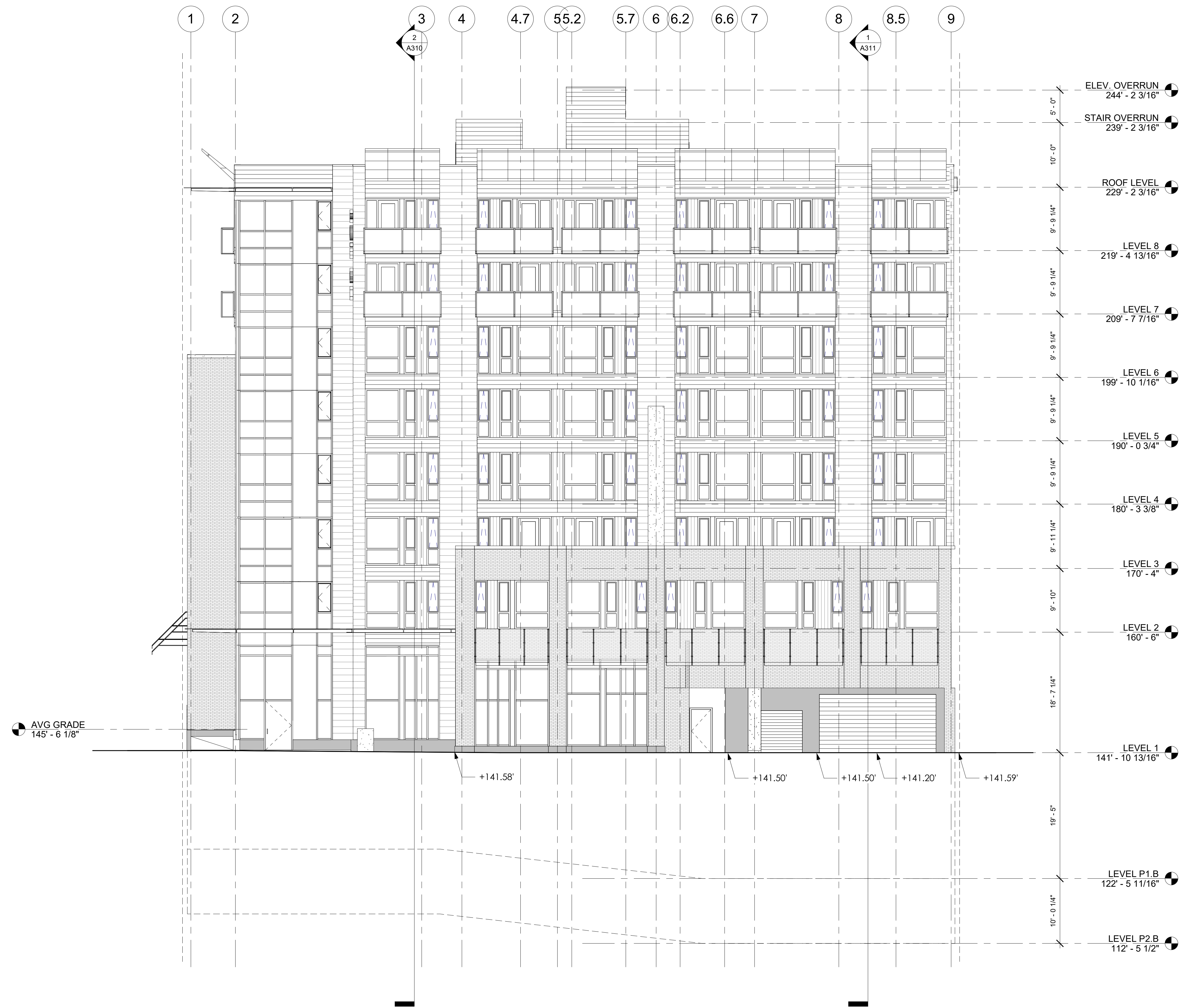
1 A303 ELEVATION VIEW - WEST SCALE: 1/8" = 1'-0" 0 4' 8' 16'
