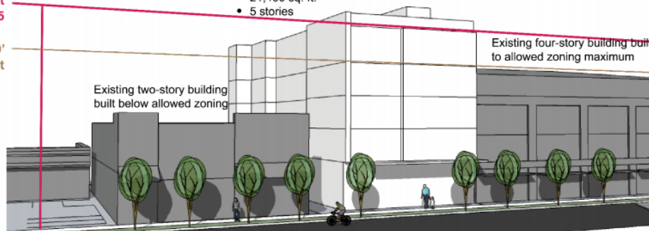
City of Seattle diagram illustrating how MHA would allow the addition of a fifth floor to a four-story building in exchange for the provision of three below-market-rate units or an in-lieu fee payment in the range of $300,000 to $400,000. A measure of development intensity, FAR (floor-area-ratio) is the ratio between the total floor area in the building and the area of the property it is built on. By City of Seattle, used with permission.
