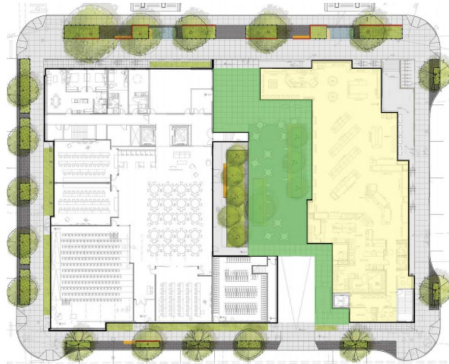
Site plan of development showing publicly-accessible courtyard and through-block connector
