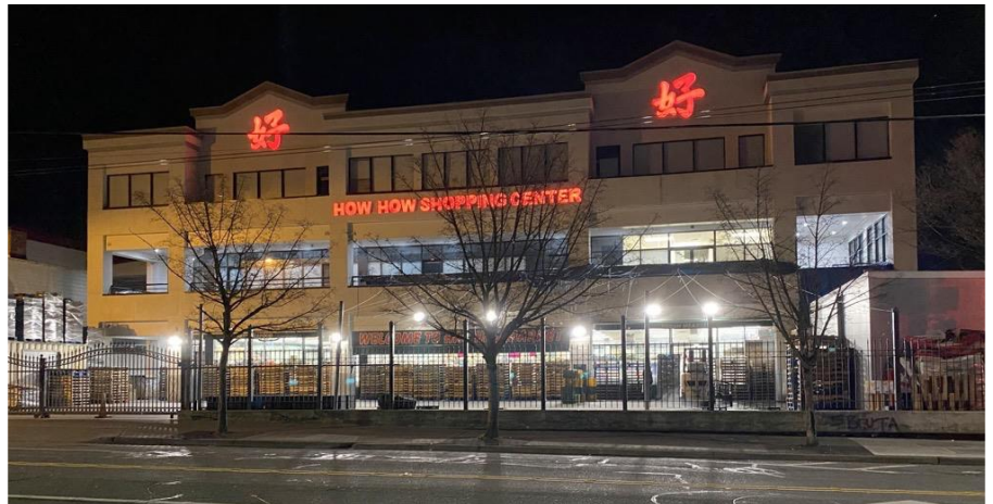
Figure 10: The How How Shopping Center is easy to spot day or night thanks to lighted signs prominently displayed above the business entrance. CPTED friendly fencing and gates allows the business owner to control access to the property and parking lot area while open and deny access after business is closed. The business is well lit, which can deter criminal activity.
