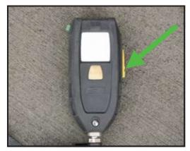
The **RESET/OFF** button (green arrow in pic.) located on the side of the unit resets the device from the full ALARM mode (2 presses). It also shuts off the unit after the cylinder valve is closed and all air pressure is bled from the unit (2 presses).
