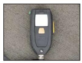
In the event that the user remains motionless for approximately **20** seconds, the ICM-Tx will enter into a pre-alarm mode. During the pre alarm mode, a RED light on ICM will flash and an audible signal will begin. Moving or shaking the ICM-Tx at this time will reset the ICM into normal operation and restart the **20** second countdown.
