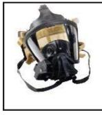
Your personal face-piece is a small, medium or large size. The lens is super-hardcoated polycarbonate and the lens has a melt temperature of 500 degrees  $F^{\circ}$  to meet NFPA 1981 standard. Applications have shown these to soften and lose structural integrity when prolonged exposures around 300+ degrees  $F^{\circ}$ . are encountered. An inhalation check valve keeps ambient moisture outside of the mask mounted regulator. The exhalation valve is a pressure demand type designed
