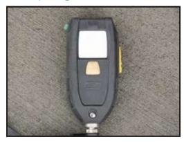
The ICM-Tx is an intrinsically safe, integrated heads-up display and an inline PASS (Personal Alert Safety System) device.
