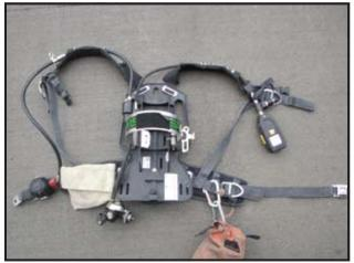
The carrier consists of a back plate, cylinder strap and latch.
