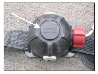
This is a pressure demand regulator, which keeps a positive pressure in the face-piece at all times. Removal of the second stage regulator by depressing the upper and lower release buttons will stop the airflow. To restart regulator, re-insert the the second stage regulator into facepiece and inhale sharply. The button automatically disengages the diaphragm, allowing air to flow to the face-piece. The
