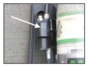
The first stage regulator keeps the pressure to the mask-mounted regulator at approximately 80 psi throughout the entire operating pressure range of the cylinder. This regulator has a redundancy feature to minimize the possibility of a first stage failure. This regulator will vent any excess pressure sent to the regulator from the cylinder.
