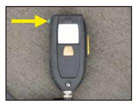
The top green **MODE** button (yellow arrow in pic) is used for unit system information. Pressing it 1 time will light up the LCD screen and refresh or relight the HUD receiver on the face-piece. While the screen is still lit, pressing the MODE button again will change the LCD screen from remaining cylinder pressure to calculated remaining service life of the cylinder. This service life number can change based on breathing/usage
