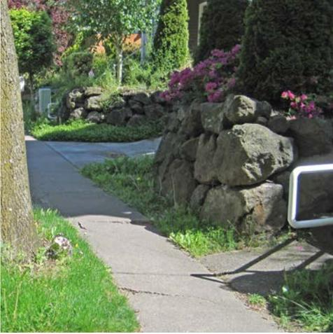
Private properties are not always at the same elevation as the adjacent public rights-of-way. A wall or rockery can be used to transition from the property to the sidewalk if the grade of the sidewalk needs to be adjusted to accommodate roots.
