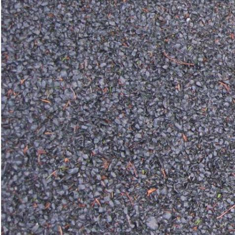
Porous asphalt is similar to regular asphalt but will allow water to pass through the pavement. It may be appropriate to use in cases where infiltration in the sidewalk pavement area is desirable.
