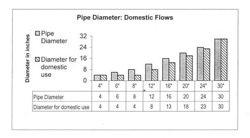
The cost of watermains is split between fire protection and domestic uses based of the shares of hydraulic capacity discussed above. The first step is to compute the installed cost for all the mains in the system.
