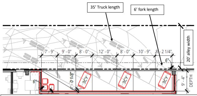
Note: The angle at which dumpsters are set out for collection depends upon the width of the alley, container dimensions, and other site-specific conditions. Trucks must be able to directly access and lift each container 24' OH and place the dumpster back down without blocking access to another dumpster.
