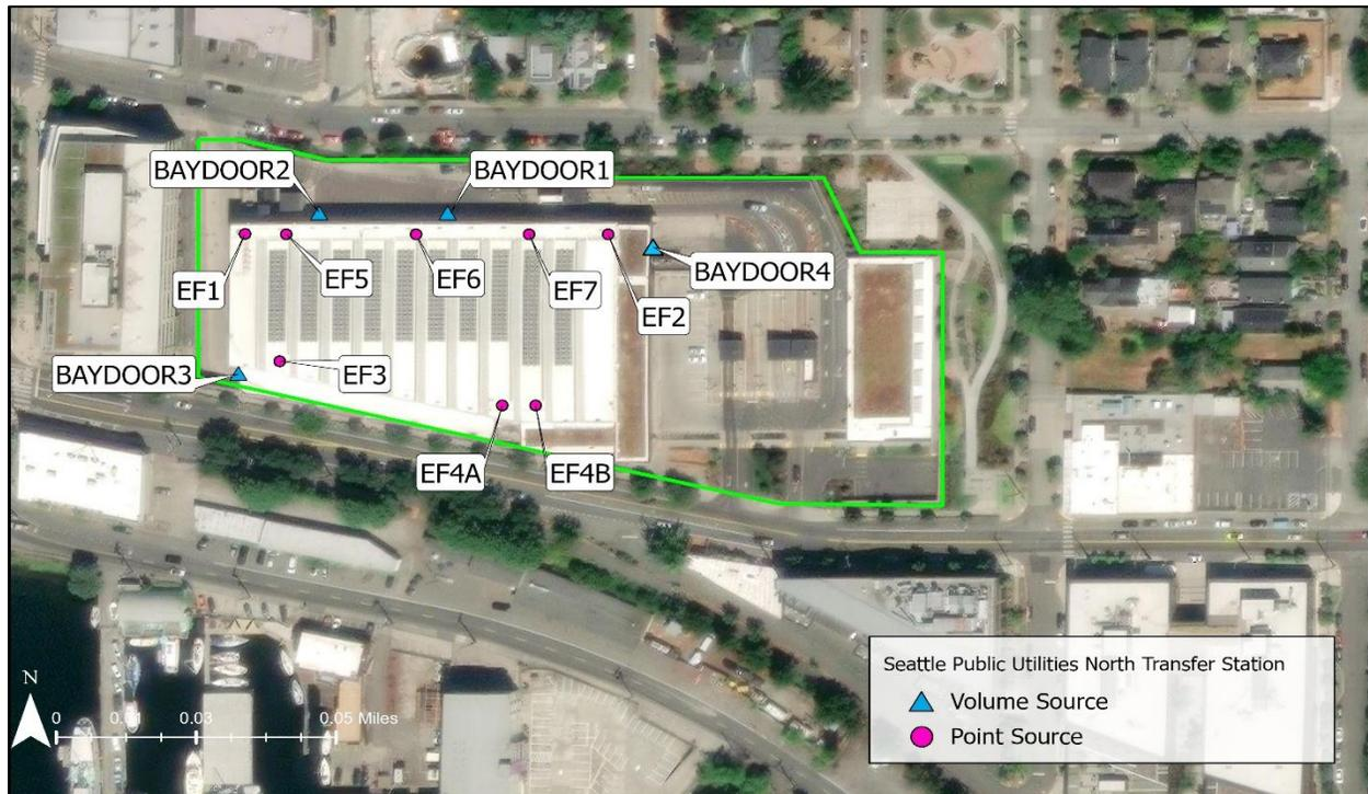
**Figure 2-1. Seattle Public Utilities North Transfer Station Identified Odor Source Locations**
