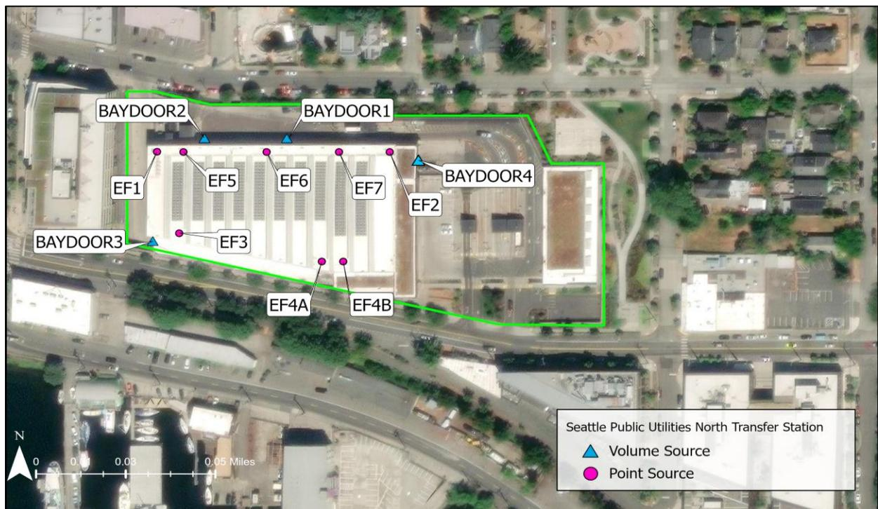
Figure 4-3. Seattle Public Utilities North Transfer Station Modeled Odor Source Locations
