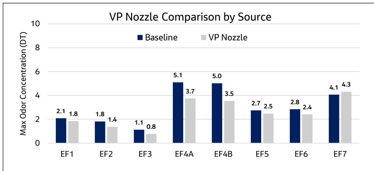
**Figure 4-6. Source Odor Impacts with Addition of VP Nozzle**
