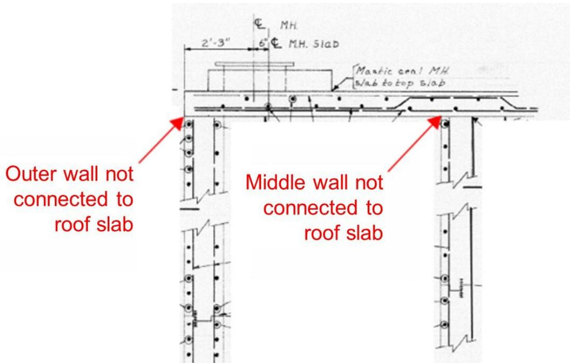
Figure E-7. Section view of PS 49
