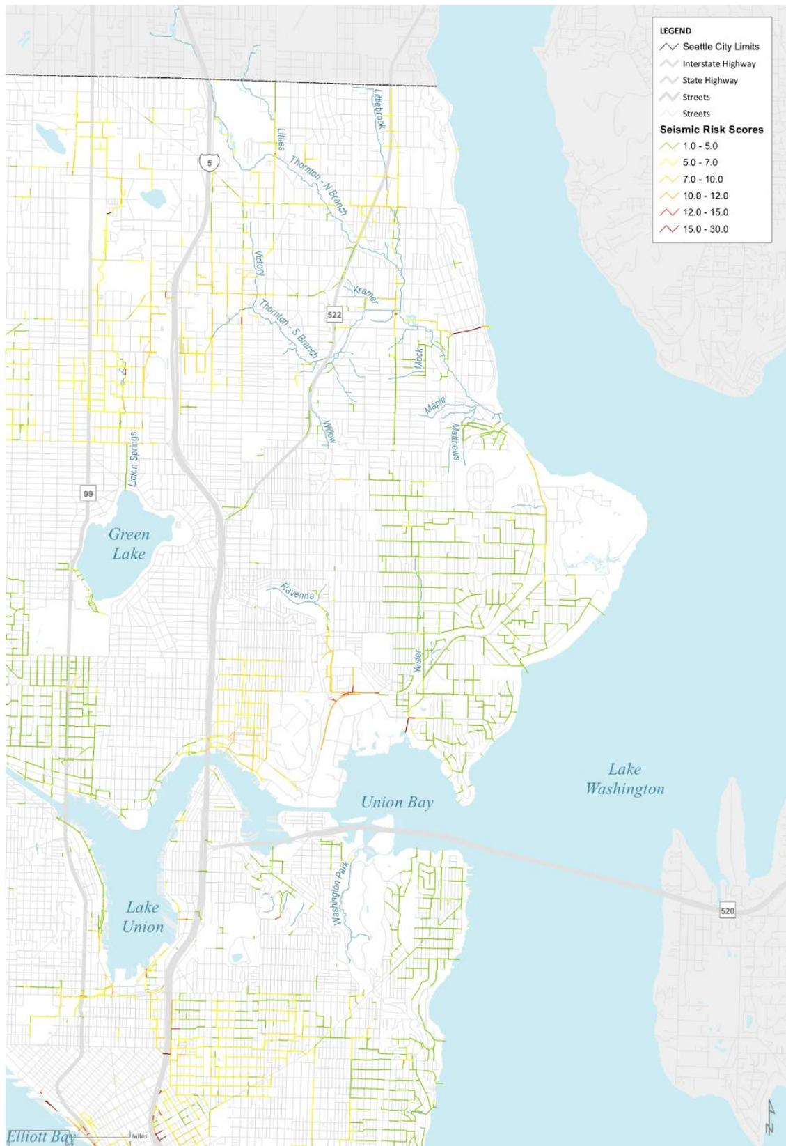
Figure 7-4. Risk scores for drainage mainlines, northeast
