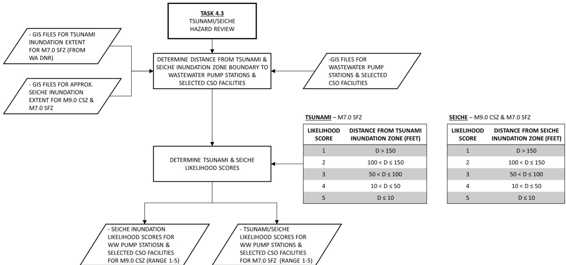
Figure 5-4. Summary flowchart for the tsunami/seiche preliminary hazards review process
