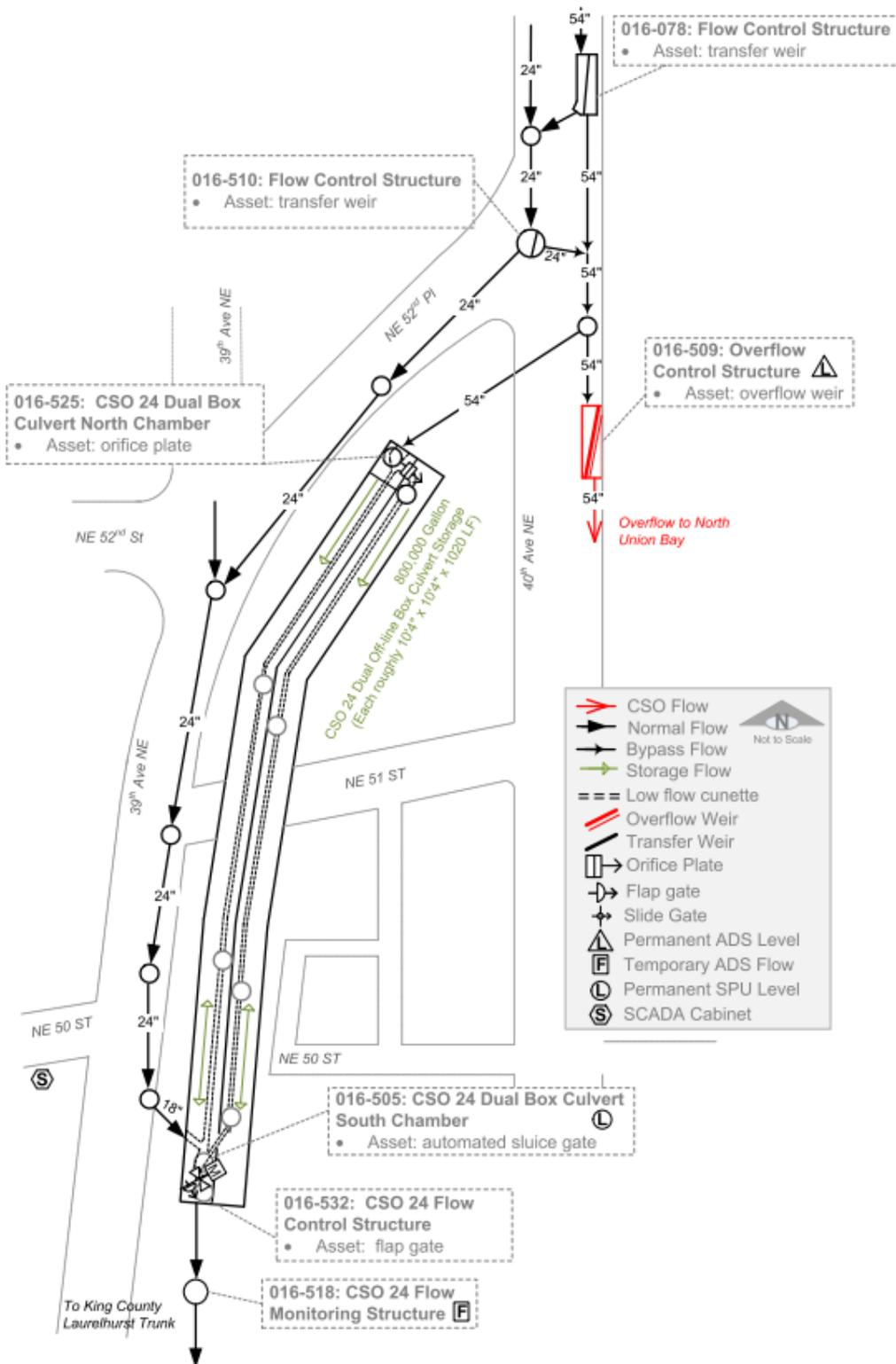
Figure J-1. Schematic for CSO 24 located between 5250 and 5130 40<sup>th</sup> Ave NE
