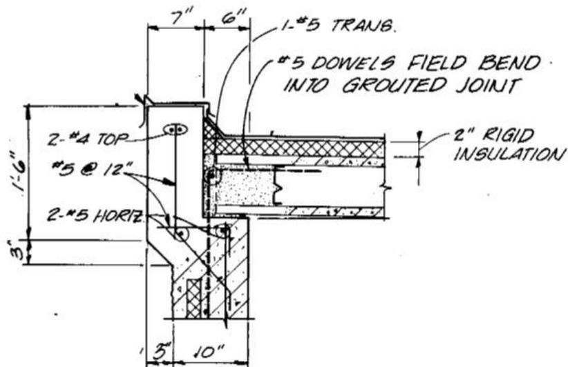
Figure E-12. Corner panel and roof diaphragm connection detail
