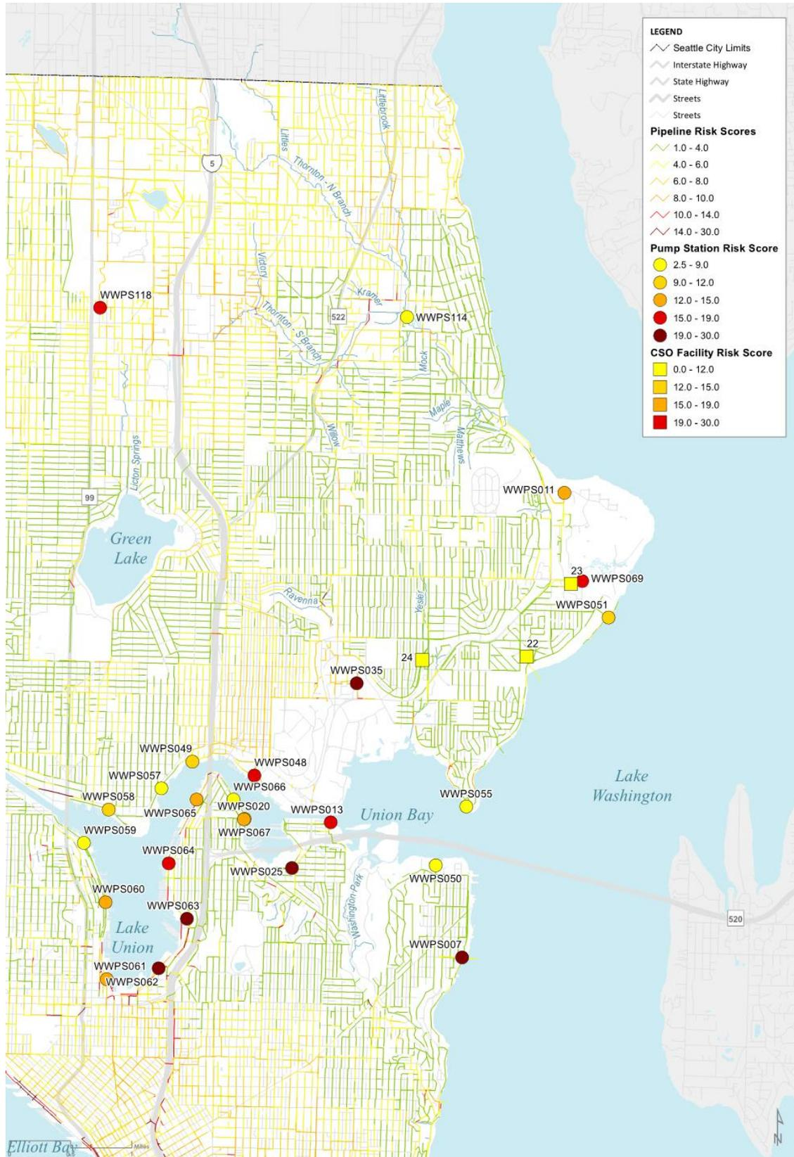
Figure 7-8. Risk scores for the wastewater system, northeast
