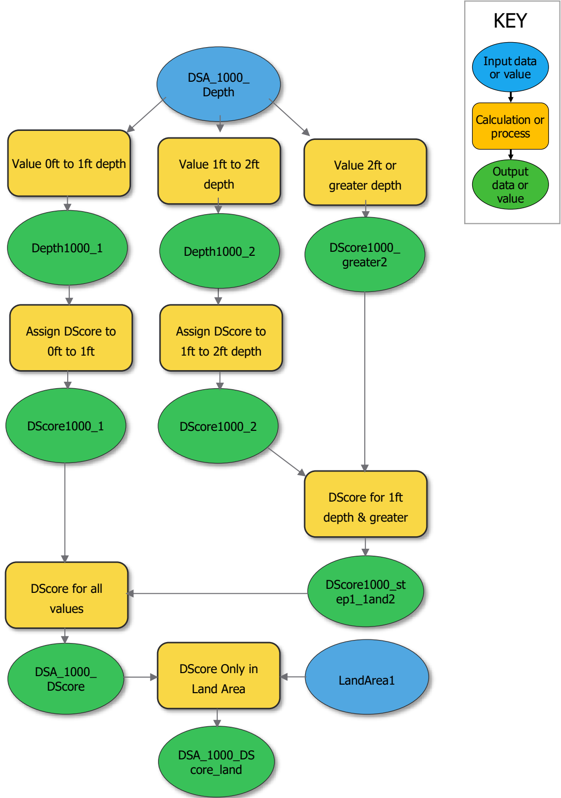
Figure B-1. ArcGIS model builder for 1,000-year inundation Depth Score
