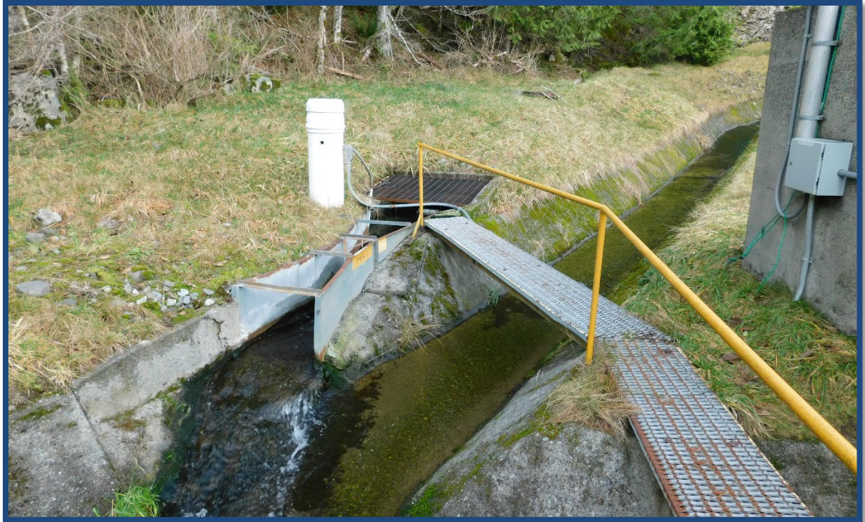
Figure 2.15 – Seepage measurement instrumentation at Tolt Dam.
