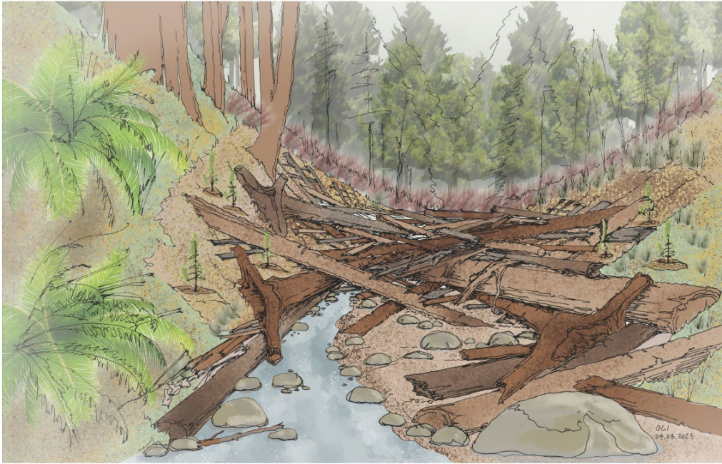
OSBORN CONSULTING INCORPORATED Taylor Creek Site 2 Station 101+50 looking upstream Machine-placed structures at installation
