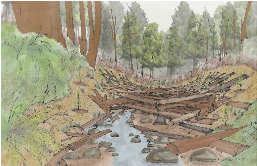
OSBORN CONSULTING INCORPORATED Taylor Creek Site 2 Station 101+50 looking upstream Manually-placed structures at installation
