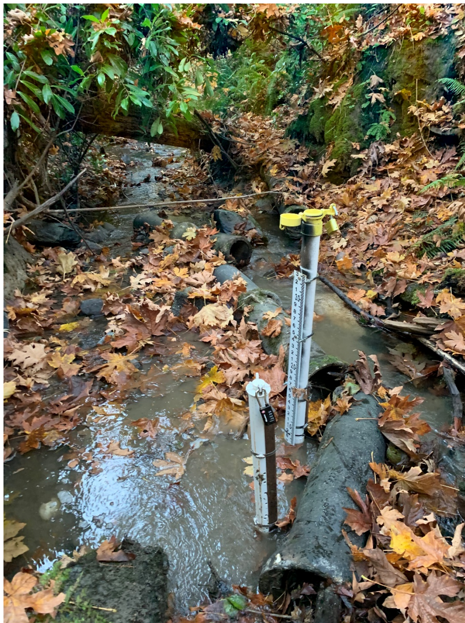
Figure 5. TC-EF Monitoring Station Showing Location of Water Level Sensor Stilling Well and Turbidimeter Stilling Well.
