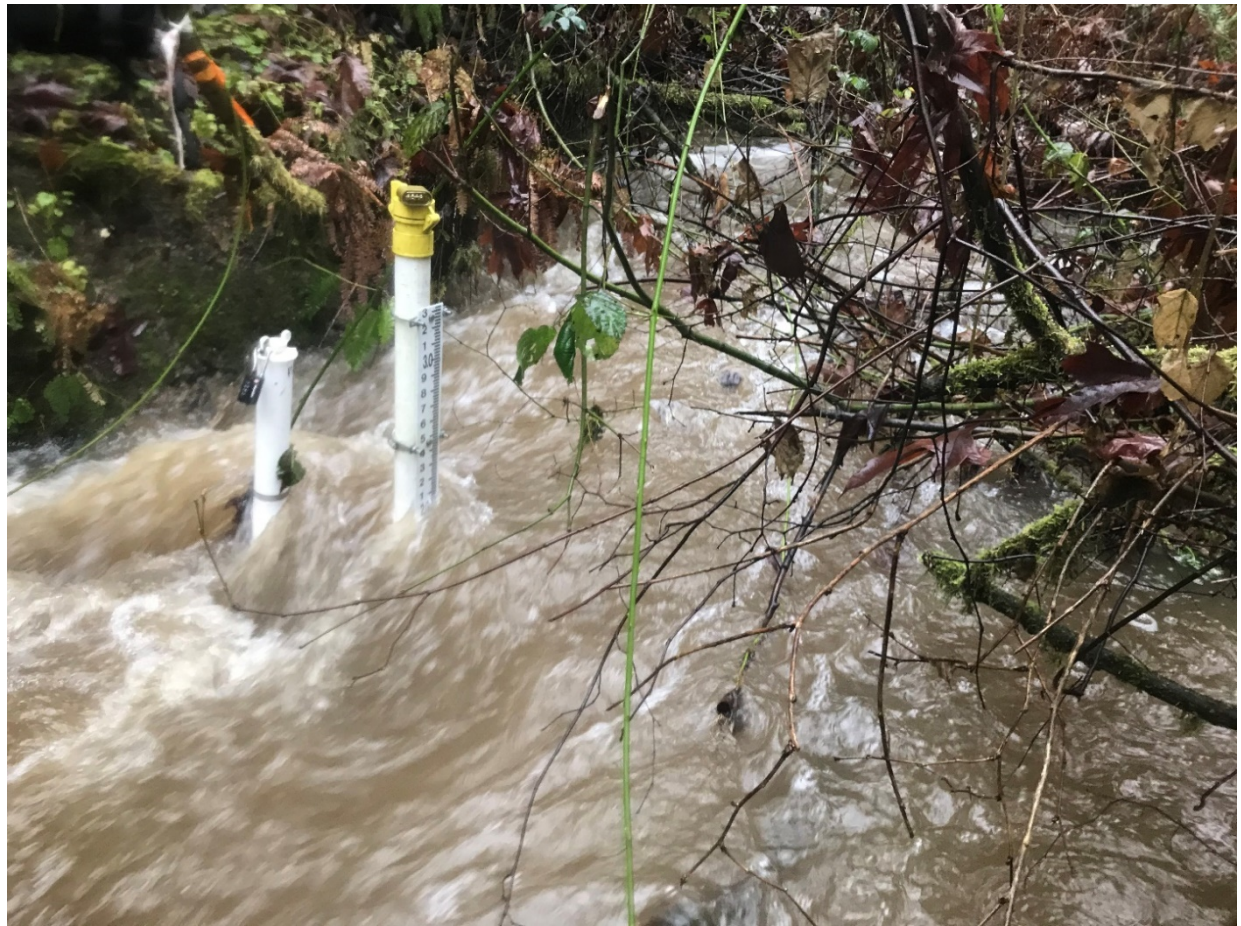
Figure 4. TC-WF Monitoring Station Showing Location of Water Level Sensor Stilling Well and Turbidimeter Stilling Well.
