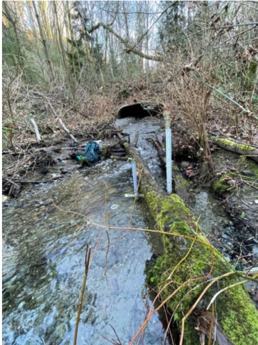
Figure 6. TC-LM Monitoring Station Showing Location of Water Level Sensor Stilling Well.
