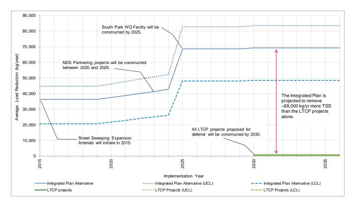
Figure 8-16. Estimated TSS load reduction benefits of the Integrated Plan
