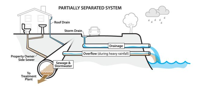
Figure 3-4. Partially separated system
