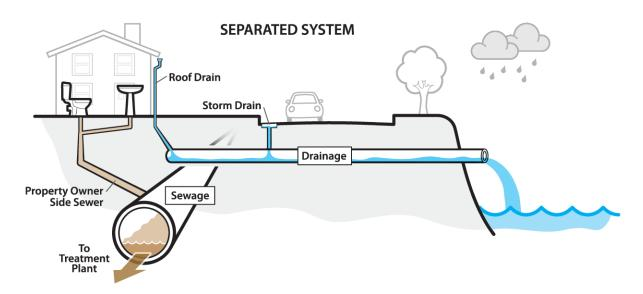
Figure 3-3. Separated storm sewer system
