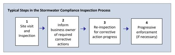
Figure II.8-2 Stormwater Compliance Inspection Process
