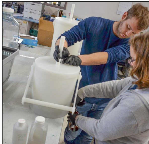
Figure 12. Compositing/splitting samples with churn splitter.
