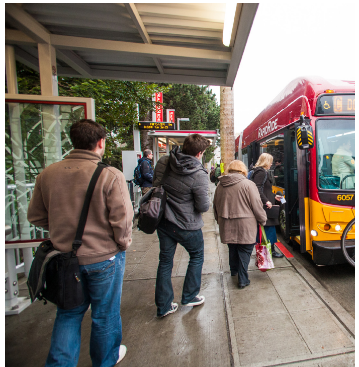
RapidRide lines C, D, and E use sixty foot articulated coaches with hybrid diesel-electric power.
