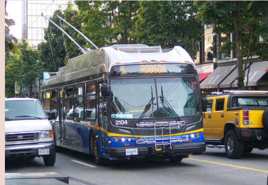
A Translink electric trolley bus in Vancouver, B.C. This is a 40' New Flyer vehicle with battery auxiliary power allowing off-wire operations.
