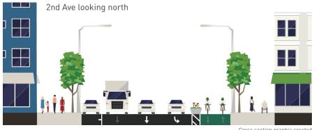
Typical cross section – with new two-way protected bike lane and left turn lane/parking lane
